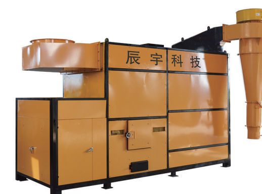
热源供给系统 Heat source supply system
